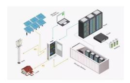
May 1, 2025 · Understanding 5kW Inverters 5kW inverters are designed to convert the direct current (DC) electricity generated by solar panels into alternating current (AC) electricity, which
