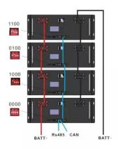
rechargeable lithium-ion batteries. It offers high energy density, long service
