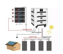
two important technologies in this domain: Uninterruptible Power Supply (UPS) systems and Battery Energy ...
