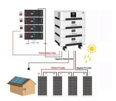
oversight of a battery pack, which is an assembly of battery cells, electrically ...
