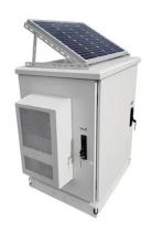
Weight 2000kg Cooling Method Smart Air Cooling Communication Port Modbus TCP?Modbus RTU?CAN2.0 Cell Type LFP-314Ah Energy 100.48kWh Rated Power 50kW Rated Voltage ...
