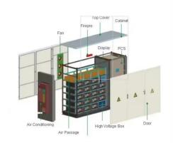
Telecom base station battery is a kind of energy storage equipment dedicatedly designed to provide backup power for telecom base stations, applied to supply
